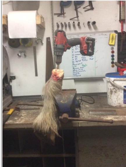
Fig 3.4 shows the position and direction of the drill in preparation of the press adaptor socket
