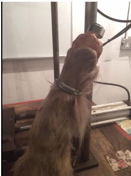
Fig 3.5 shows the press adaptor inserted and the jubilee clip that has been tightened to hold the tendons in position
